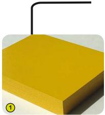
1- The painted panels are 22mm thick and made up of layers of very high quality birch which are waterproofed with a coat of phenolic resin. The edges are then sealed and 3 coats of polyurethane paint are automatically applied to each face and edge.
