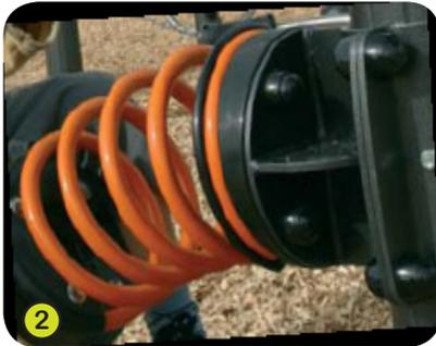
2- The **springs** are made from Grade 35SCD6 steel, shot blasted, stress relieved, zinc coated and finished with two coats of epoxy polyester powder 100 microns thick. Proludic have patented an exceptionally strong and secure polyamide fixing for the spring ensuring long product life and exceptional levels of safety.
