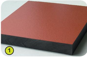
1- **The coloured panels** are made with a compact material 13mm thick. It is made up of 70% of softwood fibres and 30% of thermosetting resin, and it stands up to weathering very well (sun, rain, damp, etc.). The coloured surfaces are treated with products based on coloured acrylic polyurethane resins; this enables them to stand up well to UV radiation and resist damage.
