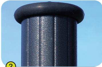
2- **The 125mm diameter posts and the 95mm square posts** are made of lacquered galvanised steel. The two-tone grey graining finish has a slightly undulating surface for increased scratch resistance. The caps are made of injection moulded polyamide.
