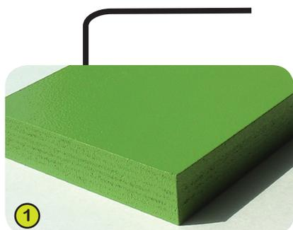
1- **The lacquered panels** are made from very high quality plywood 22mm thick. Made of alternate layers of thin birch, which offers longevity and an exceptional mechanical strength. The colours are applied by electrostatic spraying of two-component polyurethane lacquer that is free of heavy metals, to ensure high levels of resistance to potentially aggressive chemicals such as anti-graffiti cleaning products.
