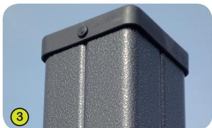
3- **The central posts**, which measure 95 x 95 mm, are made of galvanised, lacquered steel. The two-tone grey graining finish has a slightly undulating surface for increased scratch resistance. The caps are made of injection moulded polyamide.
