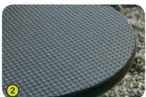
2- The table and the seats are 22mm thick panels made up of alternating layers of birch and pine. The surface is coated with a film of anti-slip phenolic resin.
