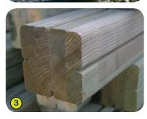
3- The 68mm square posts are made of laminated pine which has not been treated by chrome or arsenic. The laminated wood is sturdy, splinter-free and is free from shrinking or swelling. The posts are also protected from wear and tear caused by fungi, insects and termites.
