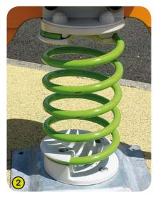
2- The springs are made from Grade 35SCD6 steel, shot blasted, stress relieved, zinc coated and finished with two coats of epoxy polyester powder. Proludic have patented an exceptionally strong and secure polyamide fixing for the spring, ensuring a long product life.
