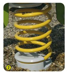
2- The springs are made from Grade 35SCD6 steel, shot blasted, stress relieved, zinc coated and finished with two coats of epoxy polyester powder. Proludic have patented an exceptionally strong and secure polyamide fixing for the spring, ensuring a long product life.
