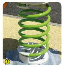
**3- The springs are** made from Grade 35SCD6 steel, shot blasted, stress relieved, zinc coated and finished with two coats of epoxy polyester powder. Proludic have patented an exceptionally strong and secure polyamide fixing for the spring, ensuring a long product life.
