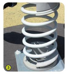
3- The spring is made from Grade 35SCD6 steel, shot blasted, stress relieved, zinc coated and finished with two coats of epoxy polyester powder.
