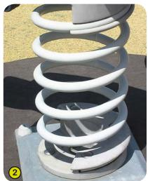
2- The springs are made from Grade 35SCD6 steel, shot blasted, stress relieved, zinc coated and finished with two coats of epoxy polyester powder. Proludic have patented an exceptionally strong and secure polyamide fixing for the spring, ensuring a long product life.
