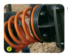
2- The spring is made from Grade 35SCD6 steel, shot blasted, stress relieved, zinc coated and finished with two coats of epoxy polyester powder 100 microns thick. Proludic have patented an exceptionally strong and secure polyamide fixing for the spring ensuring long product life and exceptional levels of safety.
